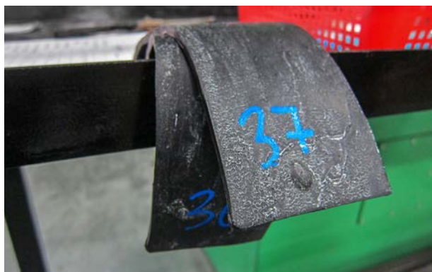
Test specimen for curemeter
